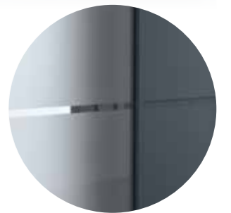
Sandblasted surface area with clear stripes
