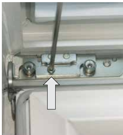
Loosen fixing screw on tilt hinge with 4mm Allen key.
