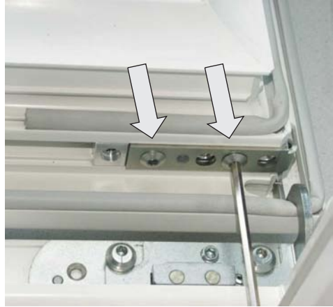
Vertical adjustment Version b Open sash max. 90°. Raise and lower sash alternately with 4mm Allen key.
